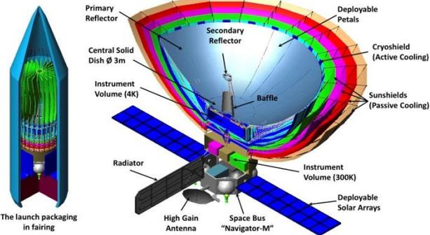
Roscosmos space telescope “Millimetron”
