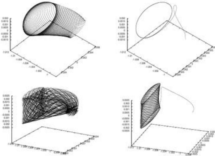
The transfer trajectory to the selected quasi-periodic orbit is searched within the invariant manifold of the restricted three body problem with help of the isoline method. This method provides connection between periodic orbit dots and geocentric transfer trajectory parameters – the isolines of transfer trajectory pericentre height function depending on periodic orbit parameters are built. This provides one-impulse transfer from LEO to the quasi-periodic orbit.
